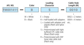
**Example:** Order number for a panel Black in color, loaded with 24 PSC adapters (4 six packs), connectors and a cable stub 10 meters in length.
