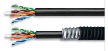
Aluminum Interlock Armor with Sunlight and Weather Resistant Polyethylene Outer Jacket (optional) Solid Annealed Copper Conductor Cross-web Separator (CAT 6 & 6A only) PFM™ Gel-filled, Water-Repellent Core Thermoplastic Insulation Sunlight and Weather Resistant Polyethylene Outer Jacket
